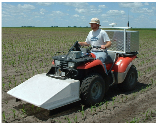
Figure 2. The ground-based corn plant population sensing system.
